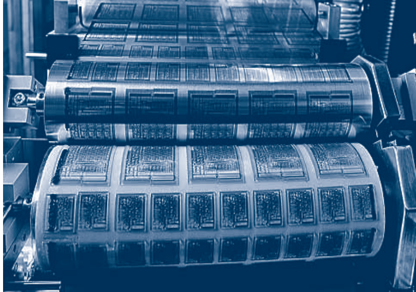
Polymer electronics printed onto a polyester film in several layers.
